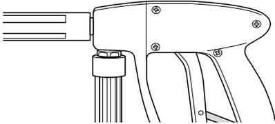
2. Safety spray gun with insulated handle and screw connection
