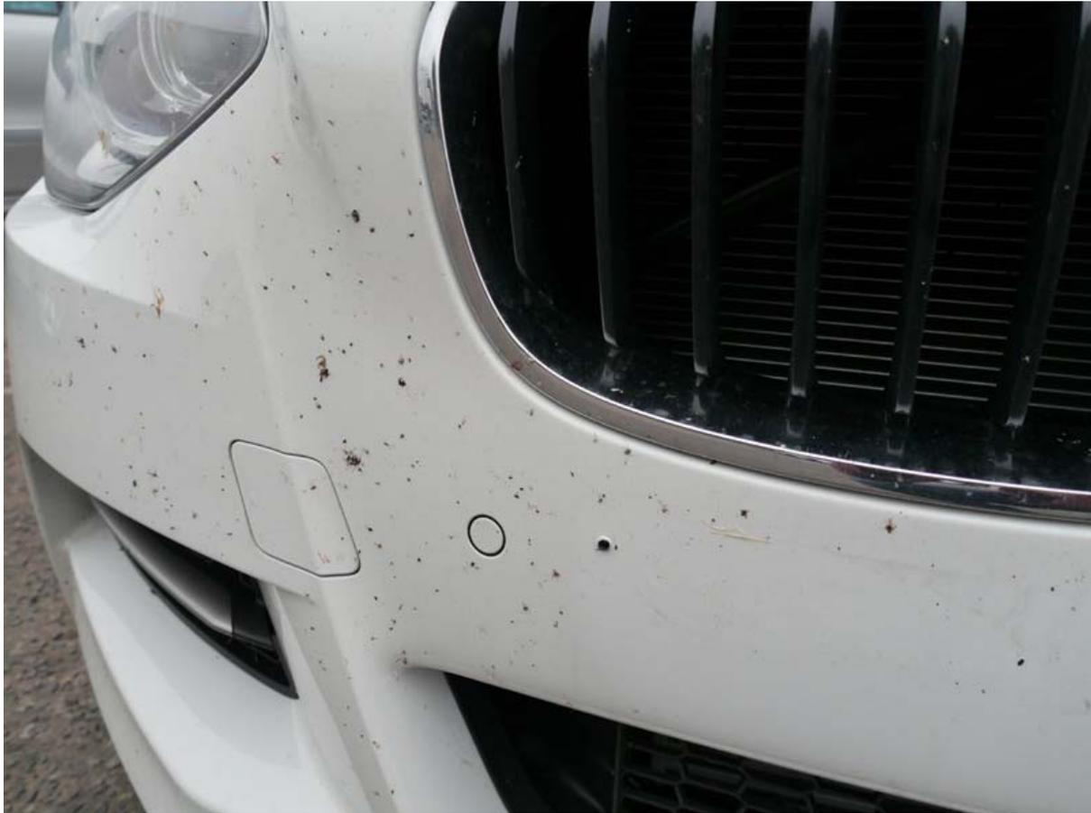
Tar, tree sap and bug residue all bond as if 'Super-Glued' to the surfaces of vehicles. There are cleaners specifically designed to tackle this type of contamination, typically called 'bug and tar removers' or 'adhesive removers'. Some of these products will turn non-painted plastic trim and window rubbers milky white and cause pitting on metals used on grilles and badges, so it's advisable to protect these first with detailing tape.
