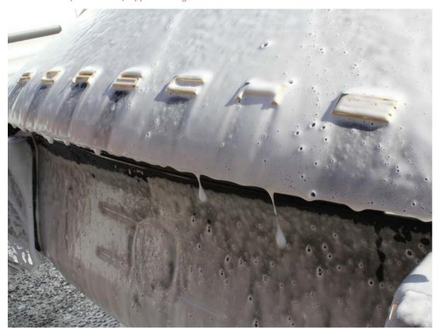
Using a pre-wash cleaner (also known as 'snow foam') applied through a foam lance connected to a pressure washer ensures the creation of thick foam able to cling to the vertical surfaces of a car for several minutes. This gives the foam maximum opportunity to get under larger particles of dirt and grit, lifting them away from the surface of the car and allowing them to be safely rinsed away.
