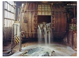
*Liming & Unhairing* - The hides are then soaked in Liming drums and treated with sodium sulphide and hydrated lime to destroy the keratinous matter. The main purpose of this process is to remove the hair from the hides. At the end of this process, the hide is usually very greasy due to a high fat content.
